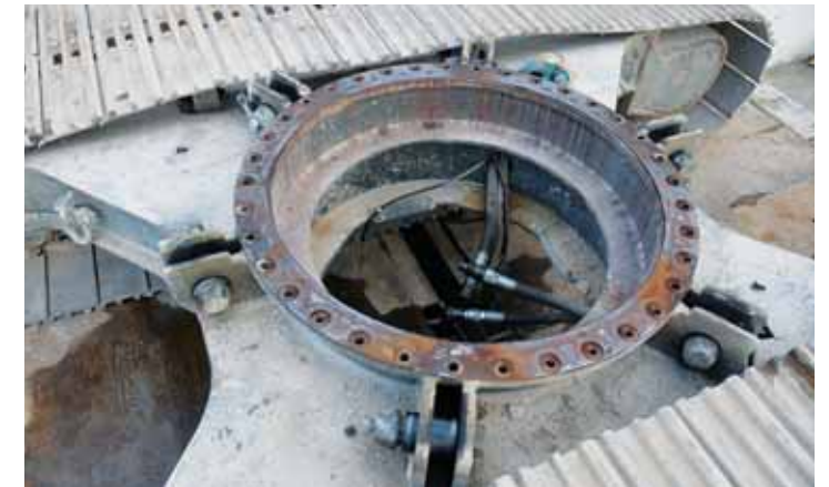
Above: The engineering works undertaken by Rusch Special Products has resulted in this cunningly-simple system to marry the two halves of the excavator.
