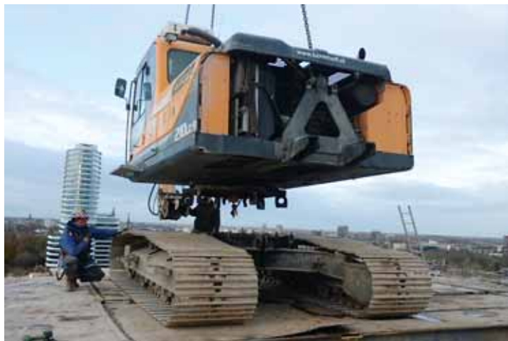
Above (Two Pictures) and Below (Two Pictures): Thanks to a quick-release counterweight and tracks, the upper-structure of the excavator is relatively simple to remove.
